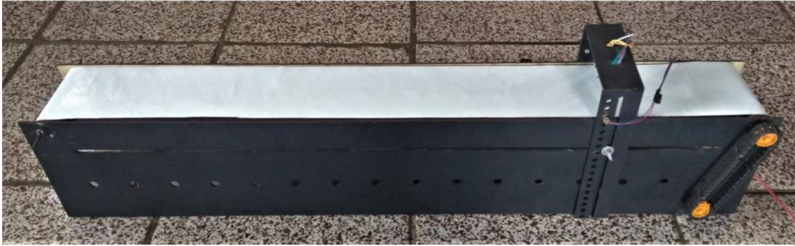
Figure 3. The developed prototype (controlled conveyor belt and sensors).
