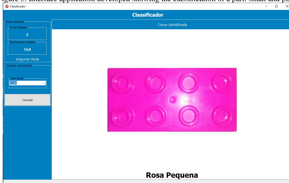
Figure 5. Interface application developed showing the classification of a part: small and pink.
