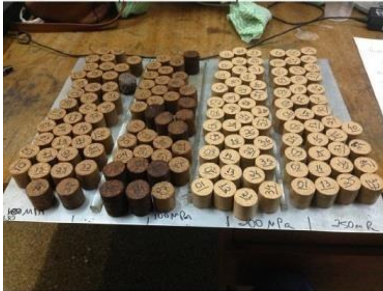
Figure 2 - Typical briquettes produced at different compaction pressures with or without the addition of carbonaceous solids.
